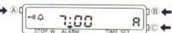
\*The alarm rings for 20 seconds. For the first 10 seconds, it beeps twice a second, and for the latter 10 seconds, four times a second.
