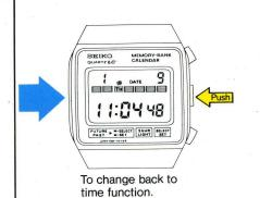
Note: To automatically advance minute, hour, etc., depress button continuously.
